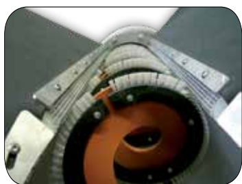
Inlet Screen Basket with Splash Guard
